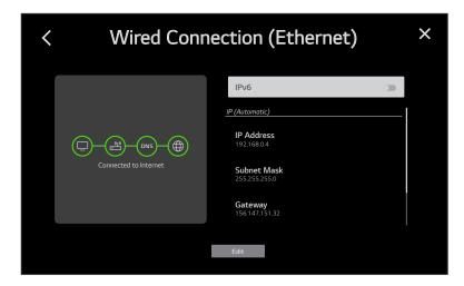
4. To enable/disable IPv6, select/highlight the IPv6 field, and press **OK** on the Installer Remote to toggle IPv6 on or off, as required.
