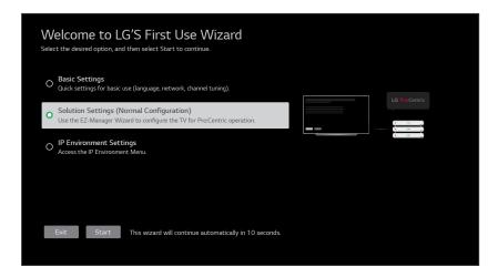
Use the arrow keys on the Installer Remote to select the desired option in the Welcome screen:
