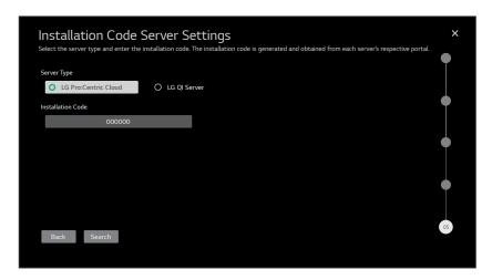
3. Use the arrow keys to select **Search** and press **OK** to verify the installation code. When the installation code is verified, the "Search" button becomes a "Next" button (you also will see a "Server Found" message below the Installation Code field). Select **Next** and press **OK** to continue.
