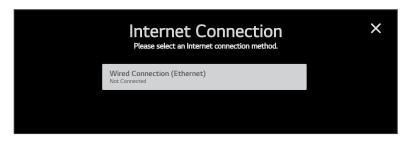
3. If the network is not configured for DHCP, or if you want to enable/disable IPv6, specify static IP configuration data (applicable only for IPv4), or change the network configuration from Manual to Automatic, select **Wired Connection (Ethernet)** and press **OK**.
