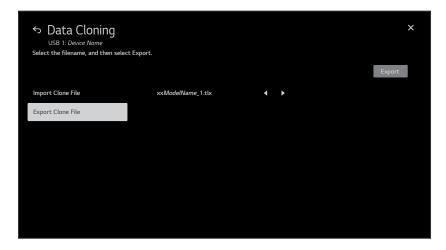
8. Modify the filename, as required. While the TV model element of the filename may not be changed, you can differentiate this Clone file from other UN560H Clone files by changing the numeric assignment appended to the end of the filename. Select/highlight the Left or Right arrow on the screen at the right of the filename, and then press **OK** on the Installer Remote to scroll through numeric assignments until the desired number is shown.
